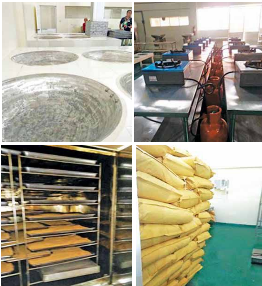
Fig. 3. Some of the facilities of the hub include (clockwise, from top left) a vat or “kawa” for cooking sap into sugar; for cooking syrup into sugar; an area for storage of the bulk processed products; and cabinet driers.
